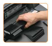
Maintenance is kept simple and minimal with just two high-yield replaceable supplies - a toner cartridge capable of 20,000 prints, and an extended life fuser unit of 200,000 prints.
