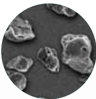
Average particle size: 8.0 micron Particle shape: non-uniform
