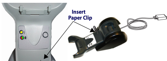
Figure 5. Disconnecting the Cable
