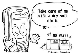
Dust or dirt accumulating on the clear plate of the reading window will affect reading performance. If you use the BHT in dusty areas, therefore, periodically check the clear plate of the reading window and clean it if dusty.
